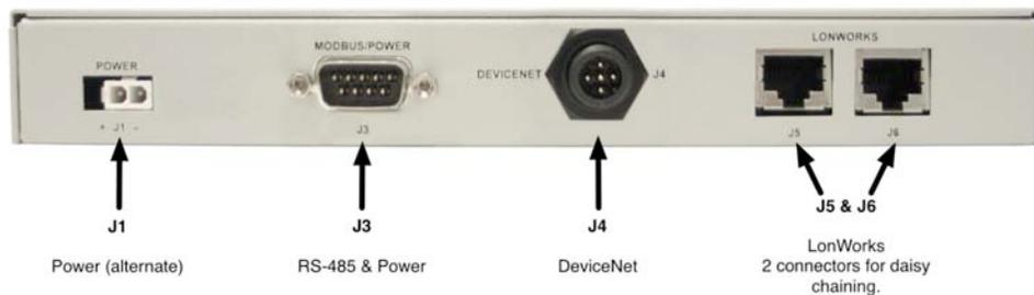
**Figure 1-3.** Rear view of the RCMe Connectors
