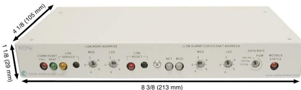
**Figure 2-1. Physical dimensions of the RCMe**
