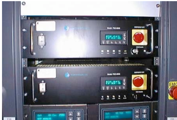
Figure 5. PSCs installed in tool's rack
